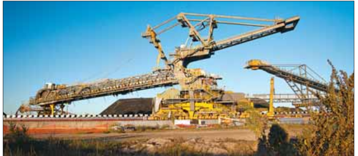
The new stacker reclaimer at the Abbot Point Coal Terminal, north of Bowen.
